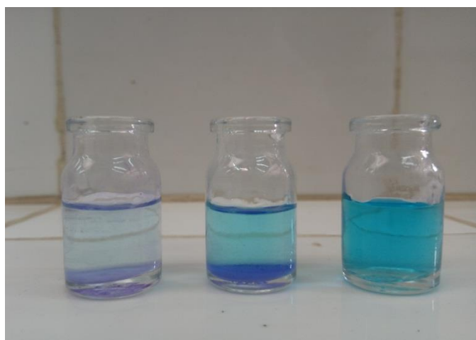
Figure IV. 20 MB solution of 3 wt. % Er-doped MgO NPs before irradiation, and after 90 min of UV irradiation exposure.
