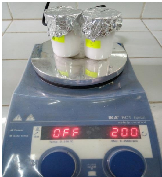
Figure II. 8 MgO solutions under magnetic stirring.
