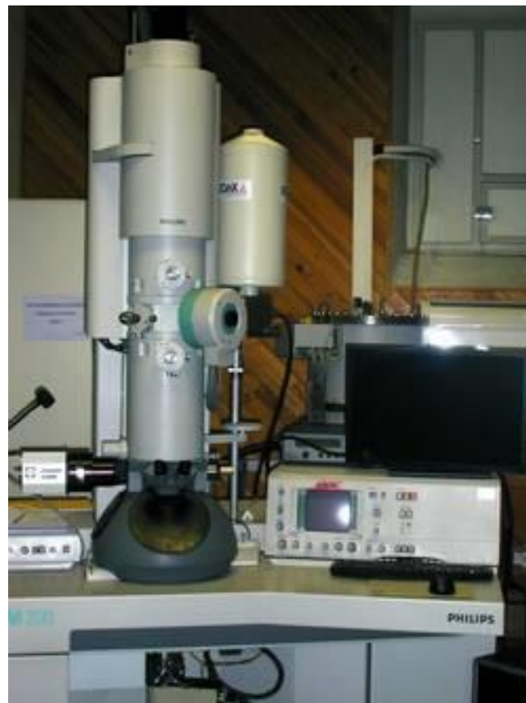
Figure II. 21 Transmission Electron Microscopy (TEM) and Energy-dispersive X-ray (EDX) type Philips CM 200 from IJL Lorraine University, Nancy, France.
