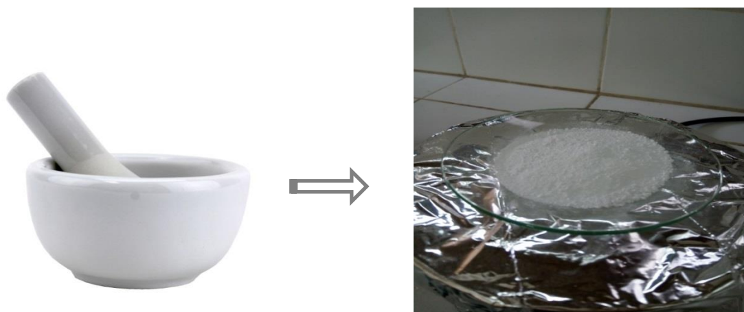
Figure II. 9 Mortar and pestle used to produce MgO fine powder.
