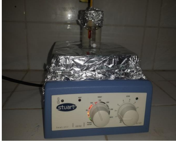
Figure II. 6 Undoped ZnO solution under magnetic stirring.
