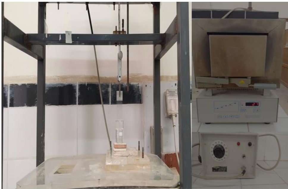
Figure II. 7 Dip-coating experiment from crystallography laboratory of Frères Mentouri Constantine 1 University.
