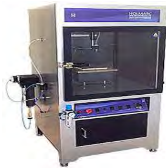
Figure II.17 The deposition system of ultrasonic spray pyrolysis (Holmarc) used for elaboration of the sensitive CuO thin film.
