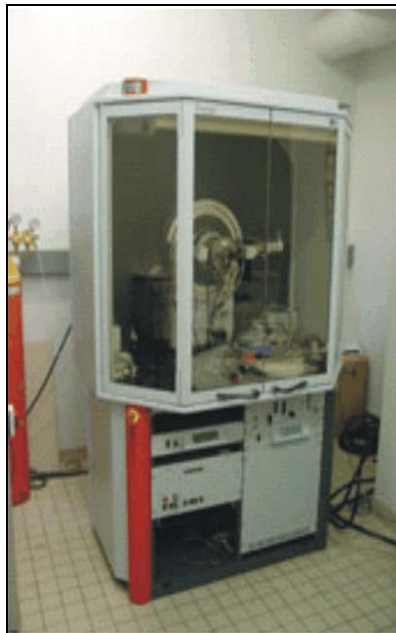
Figure III.4 : Diffractomètre: Siemens D8 Advance.
