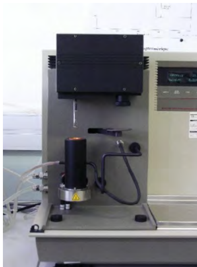
Figure II.5 dispositif ATD-ATG couplé Setsys 2400 de SETARAM
