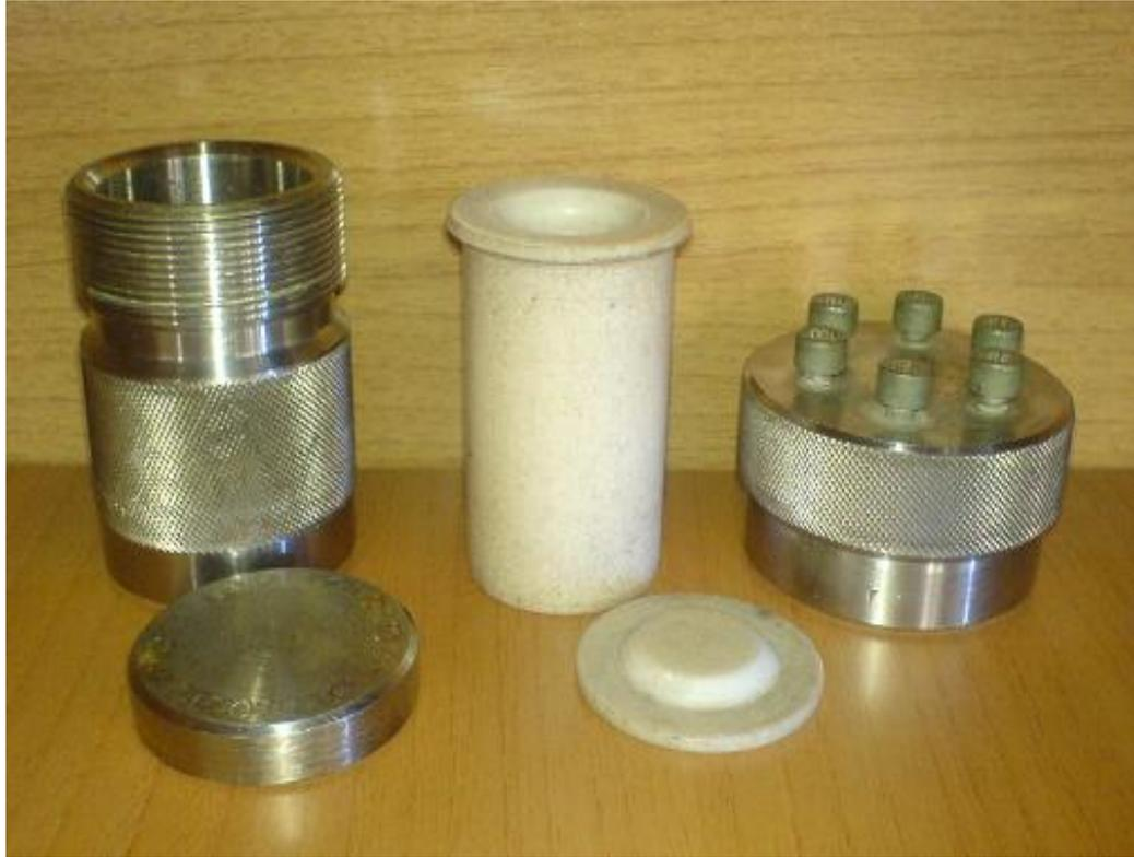
**Figure II-3 :** Autoclave locale de 23 ml.
