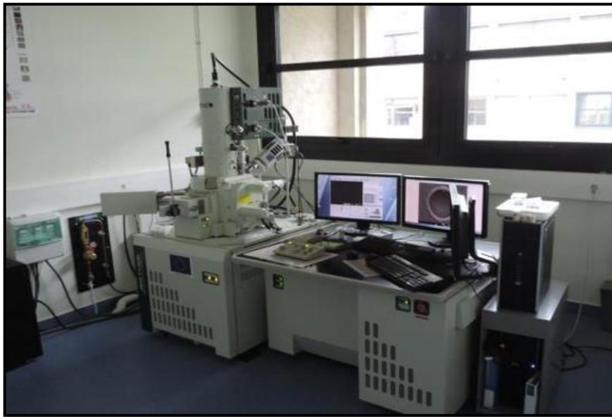
**Figure III.8: MEB-EDX "JEOL JSM 7100 F EDS EBSD Oxford".**
