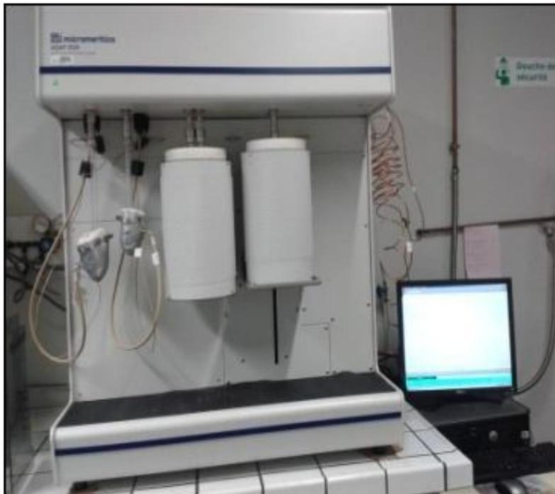
**Figure 13:** Micromeritics, ASAP 2020
