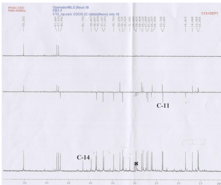
Figure IV.1.5: Spectre RMN ^{13}\text{C} et DEPT alé de LT C-7 (125 MHz, \text{CDCl}_3 , \delta ppm)
