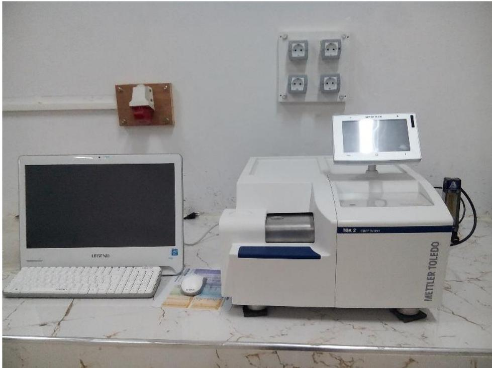
**Fig. II.16** Machine ATG model METTLER TOLEDO
