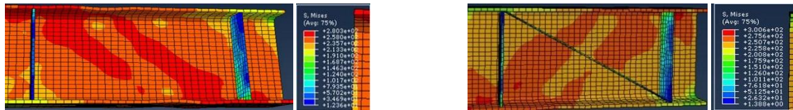
Figure 7.34. Von Mises Stress Contour of short link SL (IPE 450) a) two transverse stiffeners and two transverse stiffeners + single diagonal respectively.
