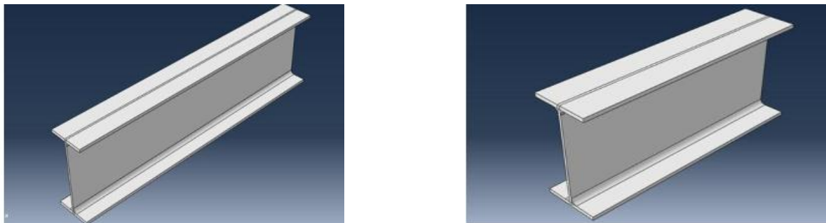
Figure 7. 23. Basic seismic link geometry configuration for long link and short link.
