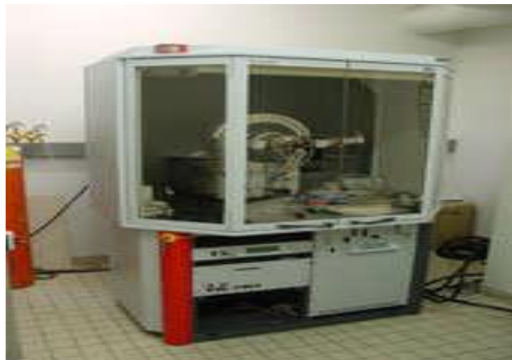
Figure III.14 — Diffractomètre de type (BRUKER - AXS type D8).
