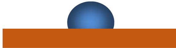
**Figure I.7** : Surface hydrophobe.
