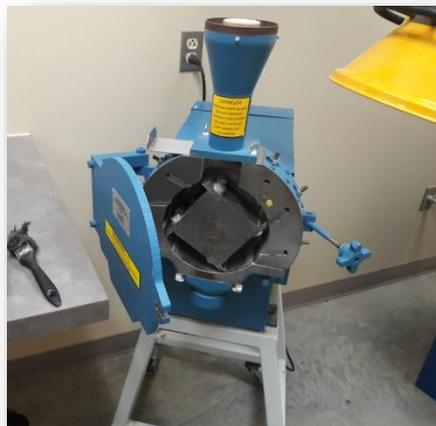
Image 5: Broyeur Wiley Laboratory Mill, Model 4 3375–E10. Nashville, USA.
