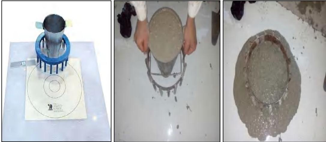
**Figure 4.16.** Essai de j-ring [85]
