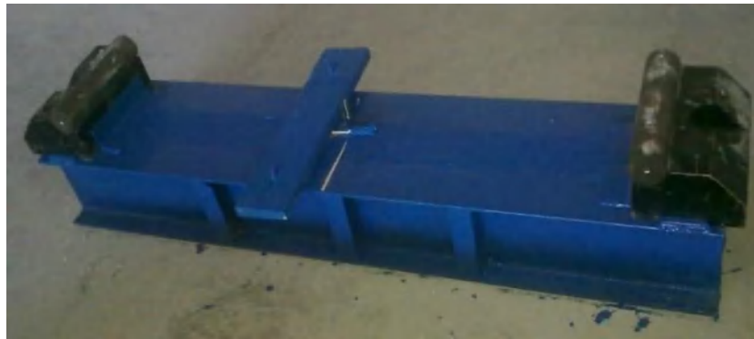
Figure (4-9): Support de la poutre
