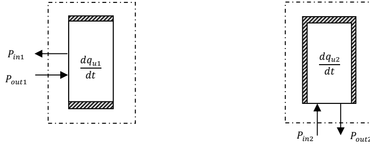
Fig.10 Boundary of the thermodynamic system, 1 index for model one, 2 index for model 2
