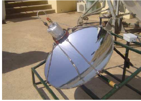
Fig.14 The solar spherical reflector used in the experiment.
