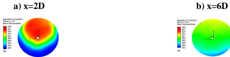
Figure 8: Contour of mean Temperature shows cross section [2D-(a), 6D-(b)] for standard T-junction.
